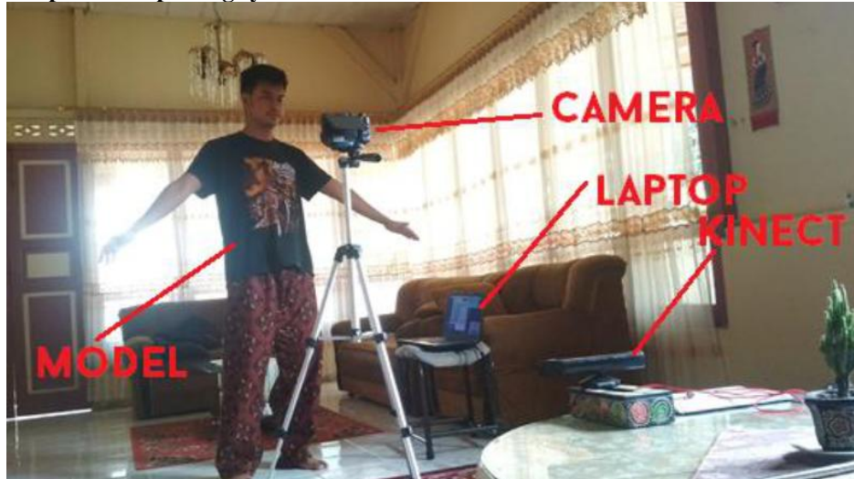
Figure 4: Components of markerless motion and posture capturing system
