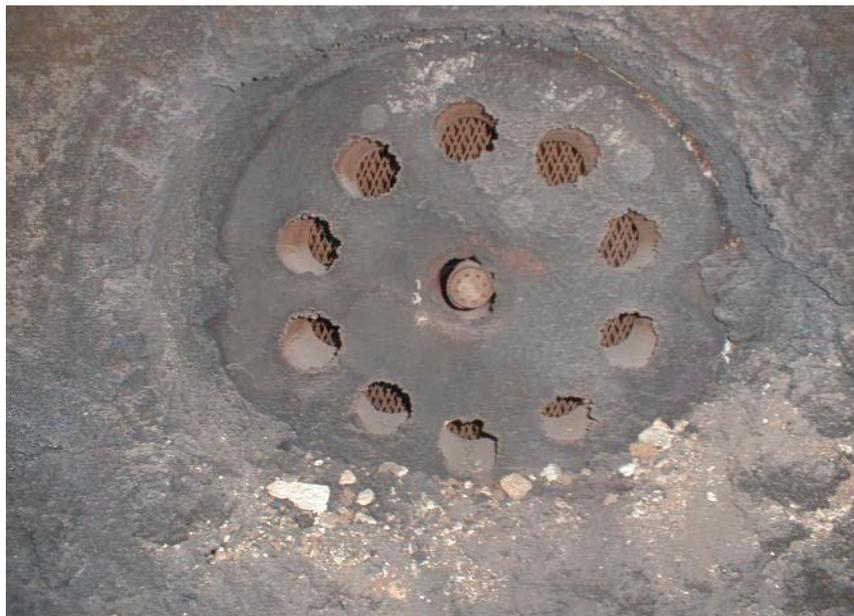
Figure 4: Scale Deposit on Buner
