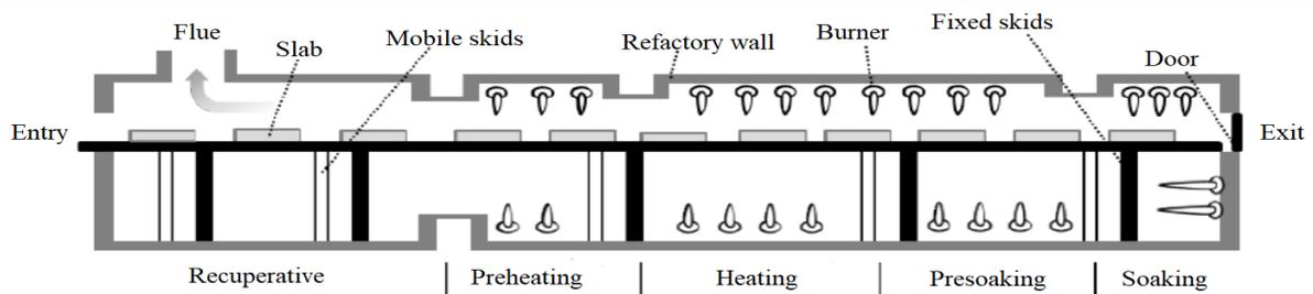
Figure 3: Typical Reheating Furnace
