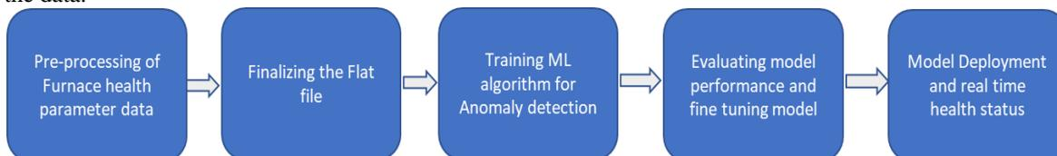
Figure 5:Process of Model Development
