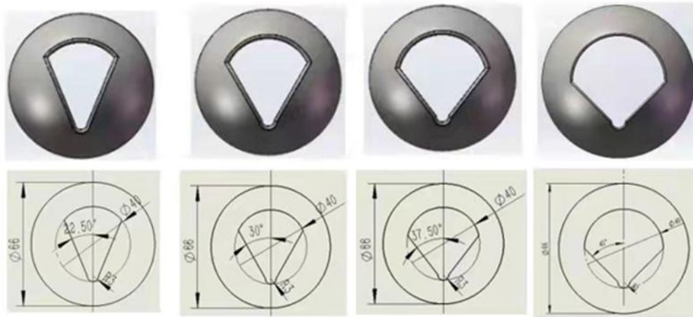
Figure 1: Four DN50 V-ball valve designs with V-shaped opening angles of 45°, 60°, 75° and 90°
