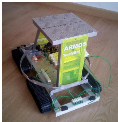
Figure 3: ARMOS TurtleBot 1 robotic platform. The robot has four tracks, each driven by a DC motor. It has WiFi communication capacity, and a control unit commanded by a Cortex A53 processor at 1.2 GHz
