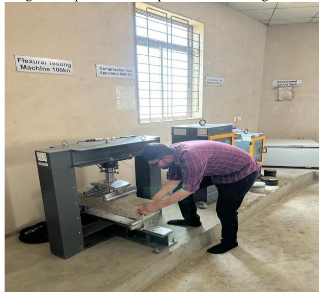
Fig. 4.4 Experimental setup for flexural testing machine
