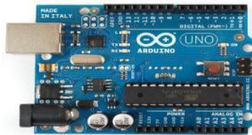
Plate I: Arduino Uno with ATmega328p Microcontroller.
