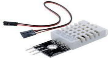
Plate III: DHT22 Temperature and Humidity Sensor
