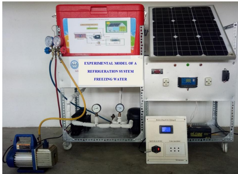
Figure 4. Experimental model of a refrigeration system freezing water
