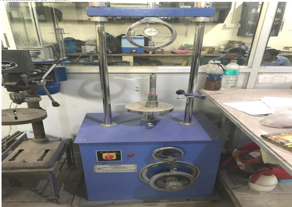
Photo 1: CBR Testing Machine
