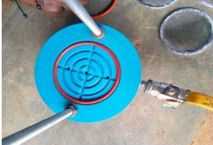
Figure 7: the drainage base
