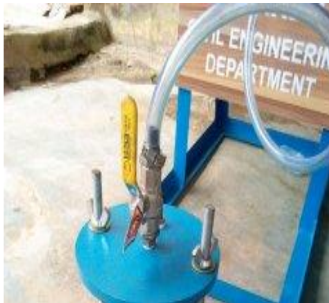
Figure 8: the drainage cap
