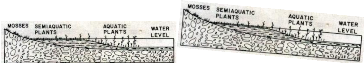
Figure 1. Formation of Coal (a) In situ method (b) Drift method
