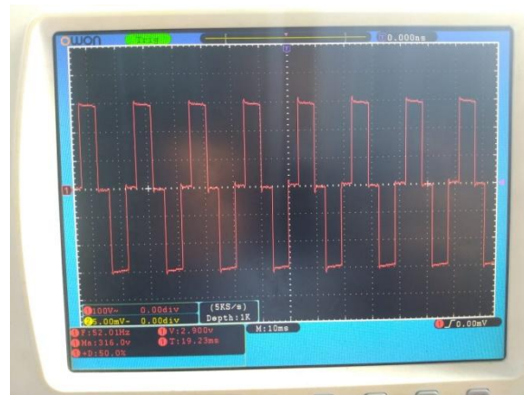
Figure 5: Single phase DC to AC inverter output waveform
