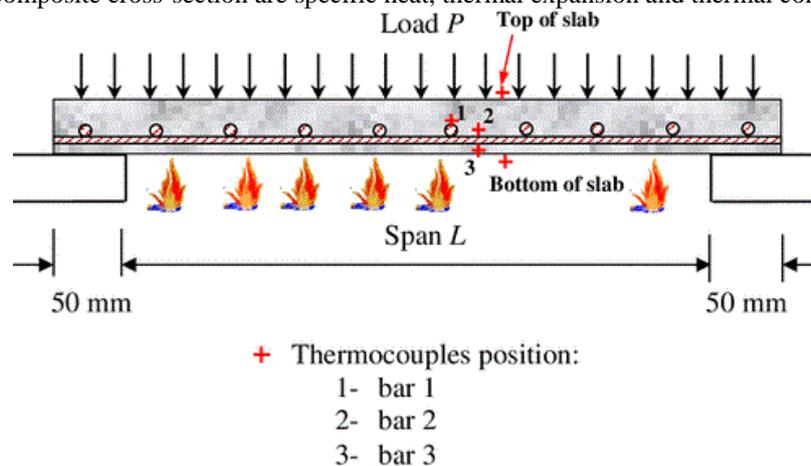
**Fig.1** Description of slab against fire
