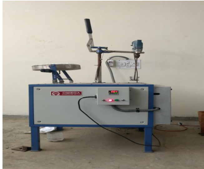
Fig 2.0 STIR CASTING SETUP
