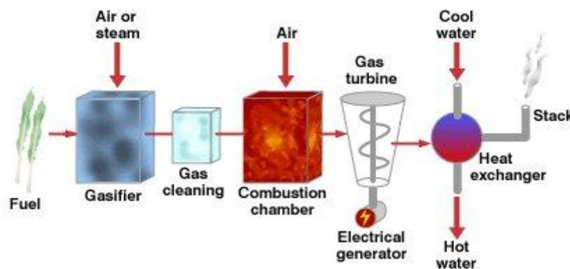
Figure 1. Biomass transformation for electrical energy
