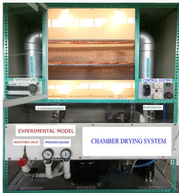
Figure 4: The experimental drying model
