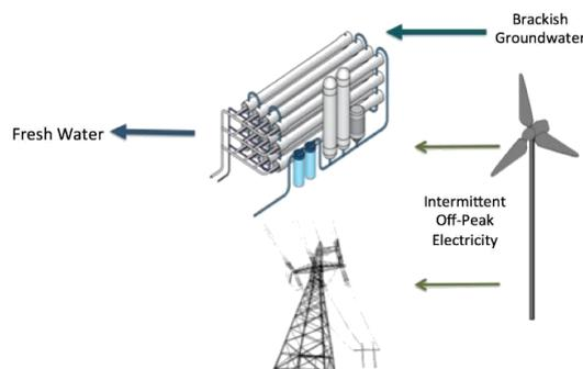
**Figure 9:** Scenario D models the traditional approach of a desalination facility that is powered by electricity purchased from the grid.
