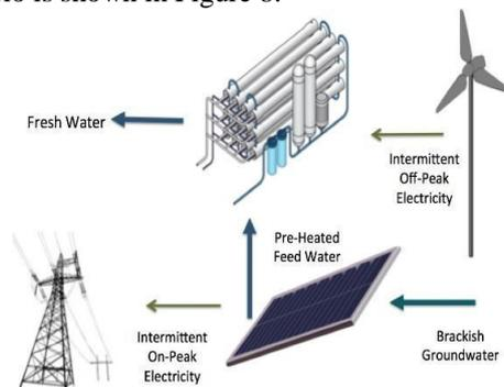
**Figure 8:** Scenario C models a desalination facility integrated with a wind farm and co-located with a solar farm. Wind-generated electricity is used to power the water treatment process while the solar panels are used to reduce the energetic intensity of desalination.
