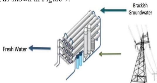
**Figure 7:** Scenario B models a desalination facility integrated with wind power that can either use wind-generated electricity for water treatment or sell wind-generated electricity to the grid.
