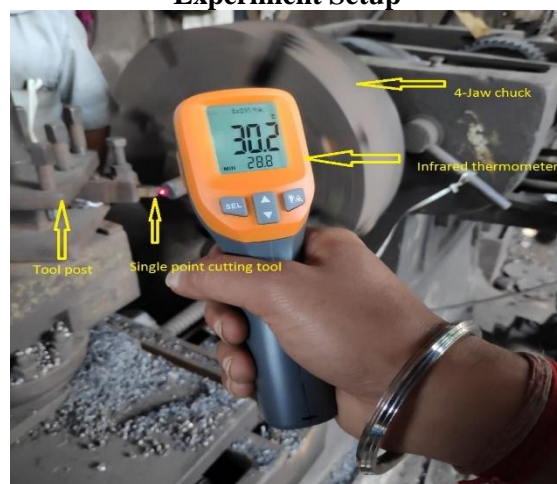
Fig. Experimental setup temperature measuring by infrared thermometer
