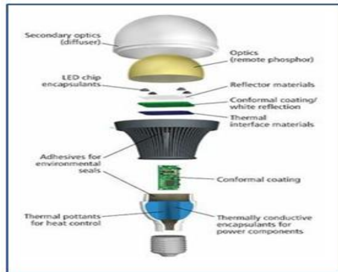
Figure 2 .Structure of LED Lamps [12]
