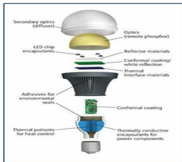
Figure 2. Structure of LED Lamps [19]
