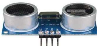
Plate V: Ultrasonic Sensor for Obstacle Detection.
