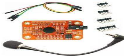
Plate I: Voice Recognition Module V3 with Connectors and Microphone.
