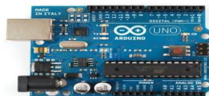
Plate II: Arduino Uno Development Board with ATmega328p Microcontroller.
