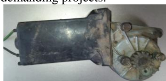
Plate III: D.C Motor for Wheelchair Drive.
