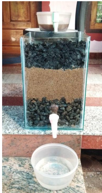
Figure 2: Filtration Set Up
