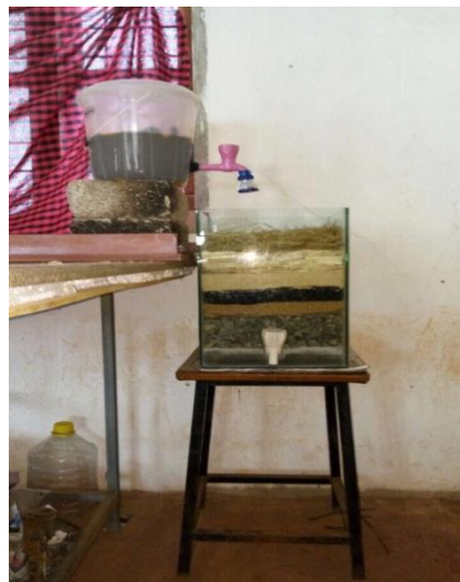
Figure: 10 Multiple Filtration Unit
