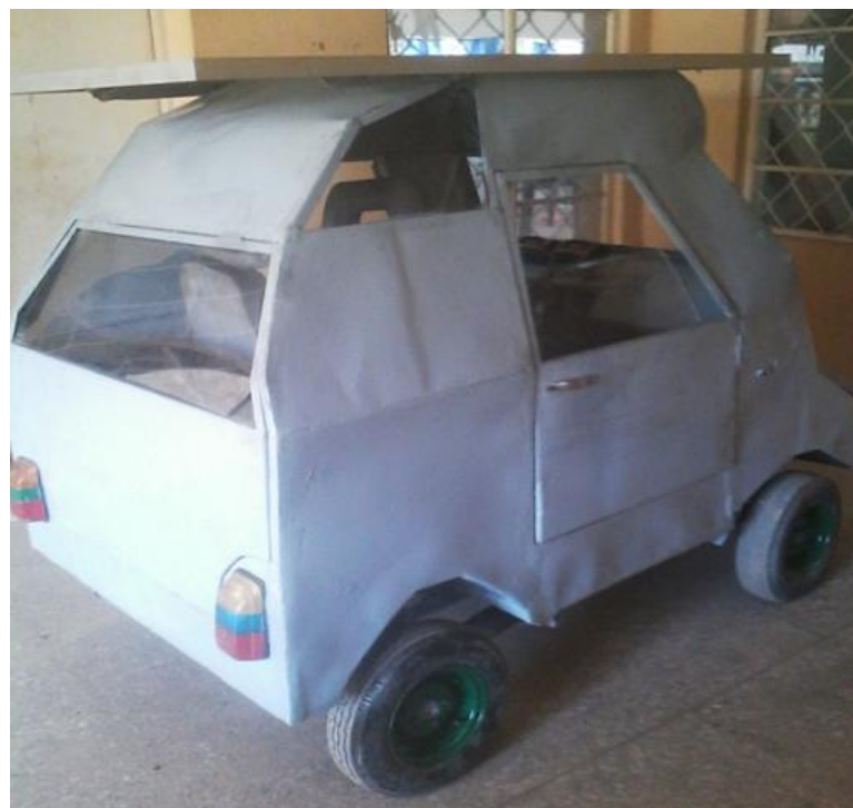
Picture 2: The Solar Panel Mounted at Angle 90^\circ on the Vehicle
