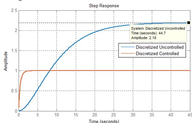
Figure 8: Response to the discretized system
