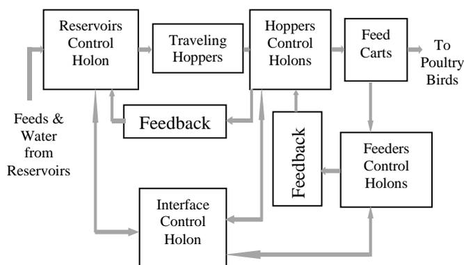
Figure 3: Block diagram of the holonic control of the automated process
