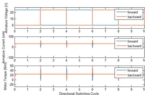
Figure 10b: Motor current and torque responses to motor driver's directional signals
