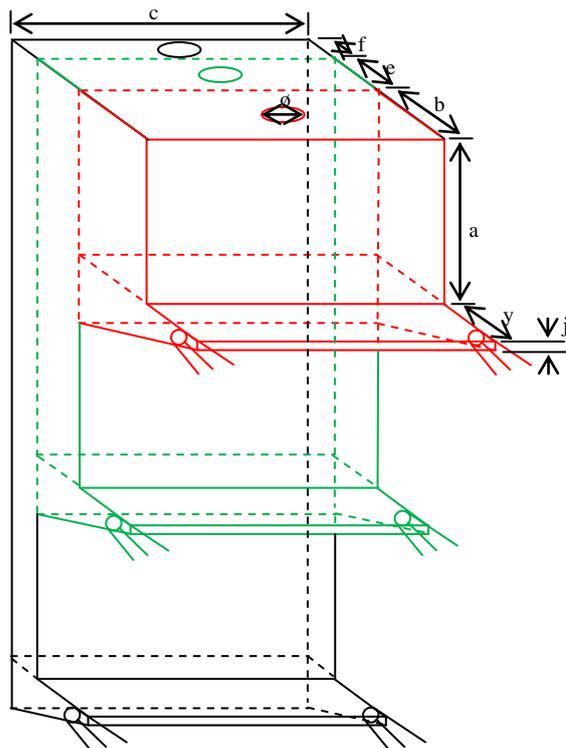
Figure 4: Schematic diagram of the travelling hopper
