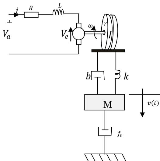
Figure 5: Motor-load model with chain and sprockets
