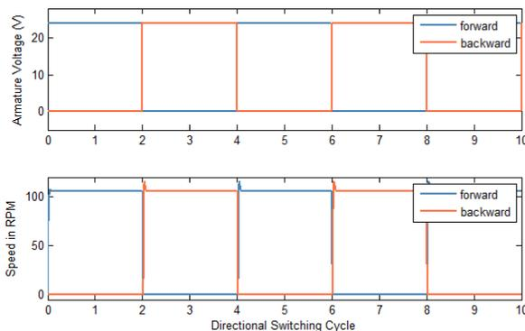
Figure 10a: Motor speed response to motor driver's directional signals
