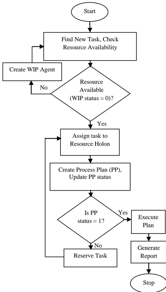
Figure 6: Flowchart for Holon Communication
