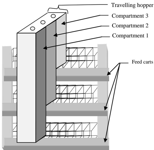
Figure 2. A section of the feeding system with the travelling
