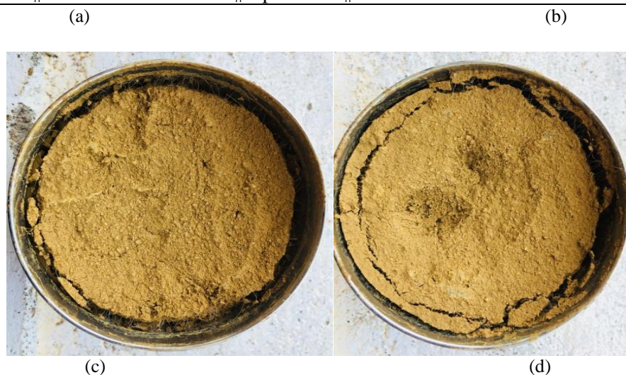
Fig.5.4.(b):Surface cracking features of Polypropylene Fiber of 6mm (a)Unreinforced Sample (b) Reinforced Sample (0.4%) (c) Reinforced Sample (0.8%) (d) Reinforced Sample (1.2%).
