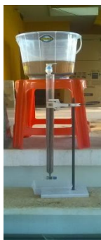
Figure 3: Adsorption Using Carica Papaya Leaf
