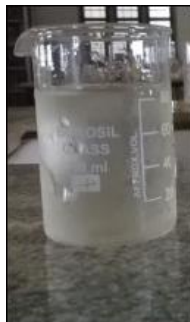
Figure 13: Treated waste water using Rice husk ash
