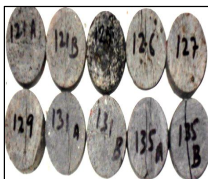
Figure 5 : Failed samples of basalt ( C )
