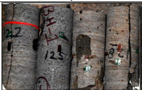
Figure 3: Failed samples of Central India basalt
