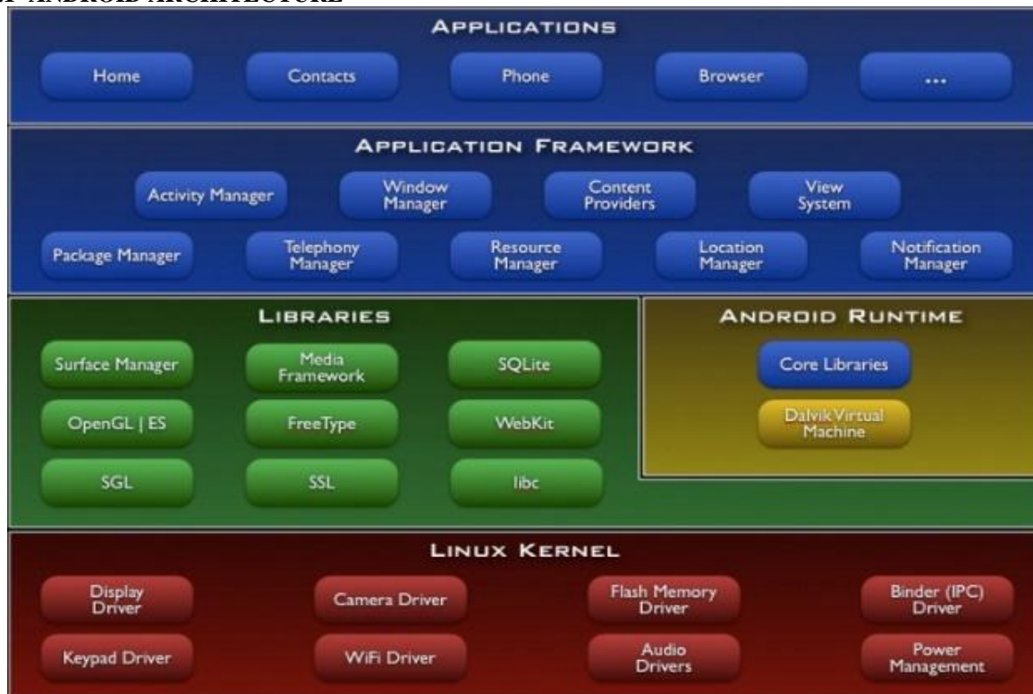
Figure 1: Android Architecture (Source: https://elinux.org/Android_Architecture )
