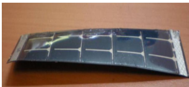
Fig. 2, PV panel colour change [114]
