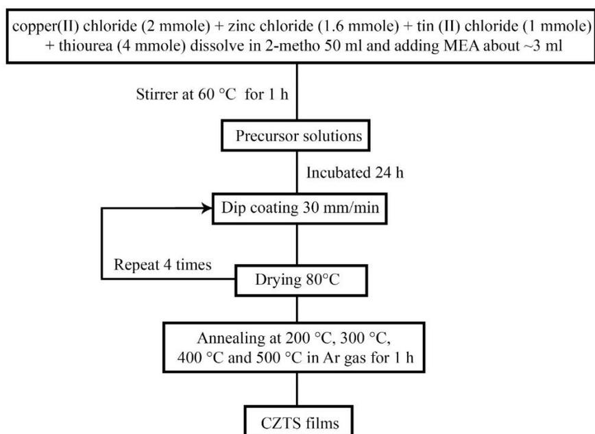
**Figure 1:** Schematic diagram synthesized of CZTS films.
