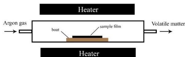
**Figure 2:** Schematic annealing process of CZTS films.
