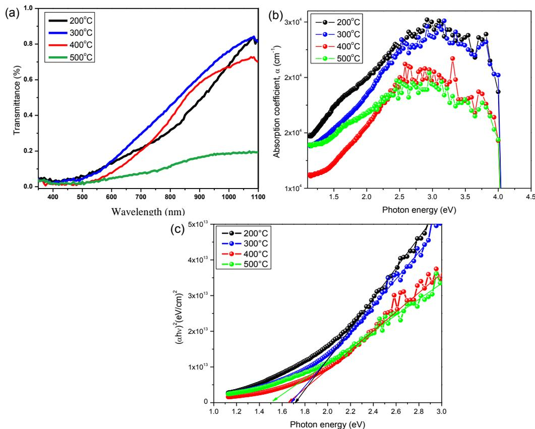
**Figure 9:** Optical properties of CZTS films annealed different temperature (a) transmittance (% $T$ ), (b) absorption coefficient ( $\alpha$ ) and (c) energy bandgap ( $E_g$ ).
