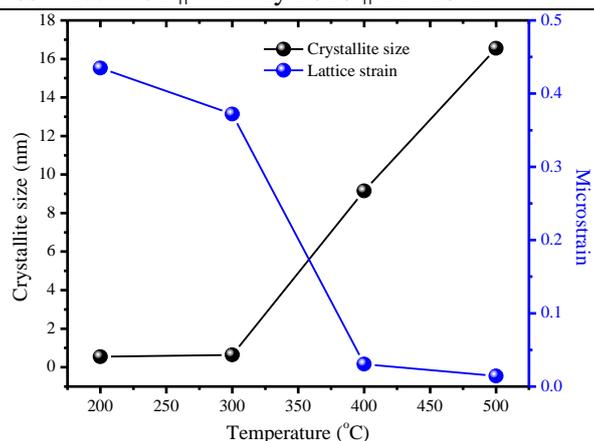
**Figure 5:** Crystallite size and microstrain of CZTS films growth by dip coating deposition.
