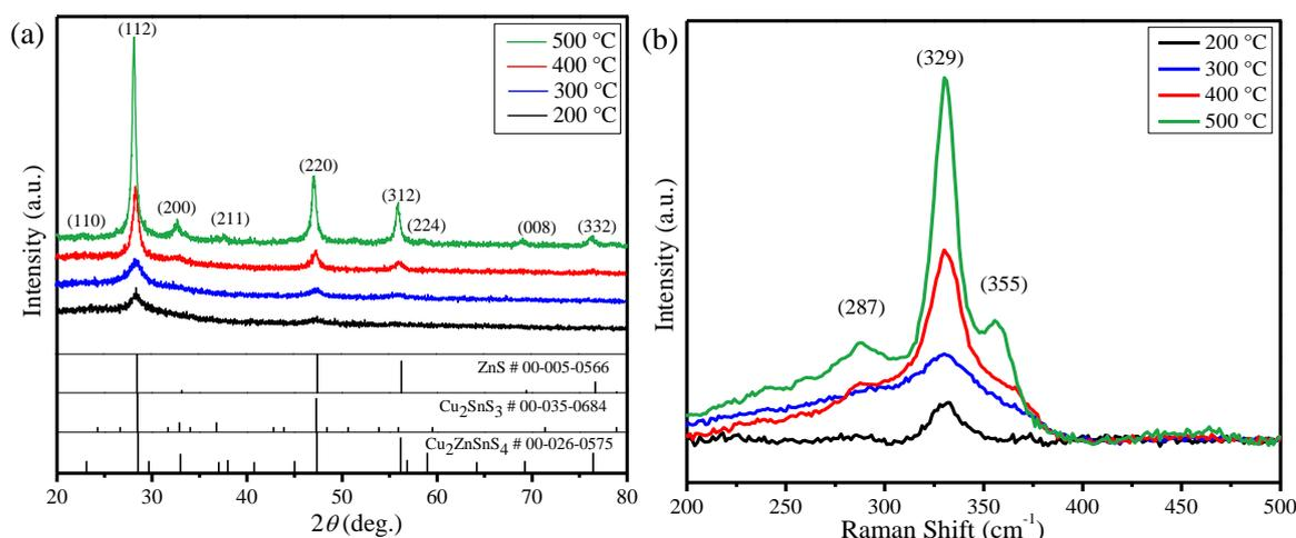
**Figure 4:** (a) XRD patterns and (b) Raman spectra of CZTS films growth by dip coating.
