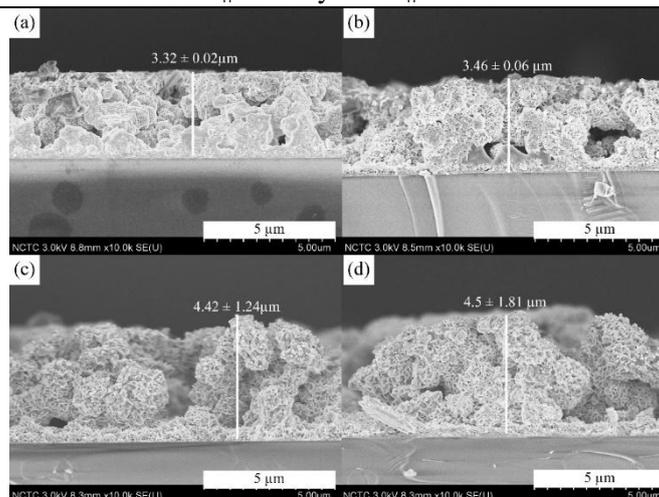
**Figure 8:** SEM cross-section image of CZTS films (a) 200°C, (b) 300°C, (c) 400°C and (d) 500°C
