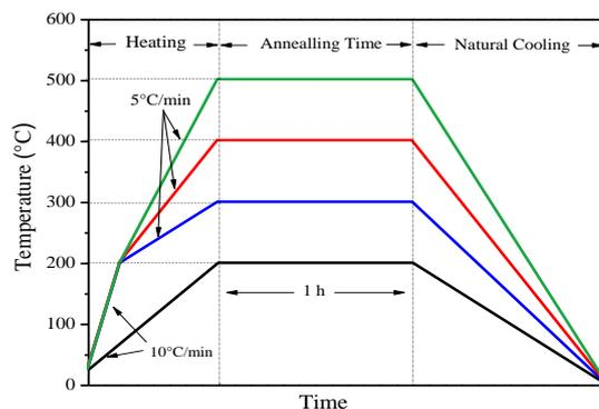
**Figure 3:** Schematic annealing temperature step of CZTS films
