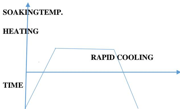
Fig 1: schematic diagram of heat treatment
