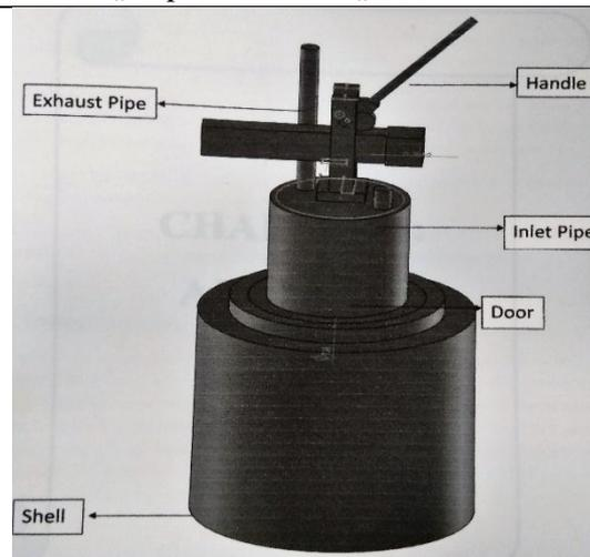
Fig: Gas carburizing furnace
