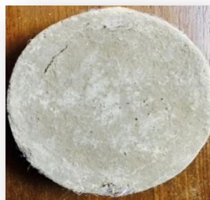
Figure 10) a. Surface cracking feature of 0% fiber
