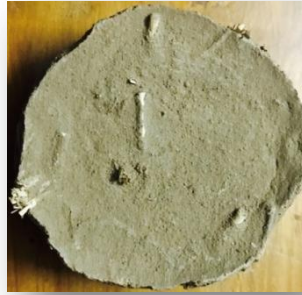
Figure 10) c. Surface cracking feature of 0.4% Straw fiber
