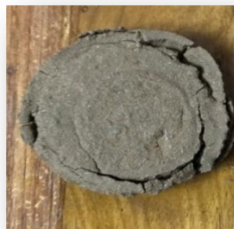
Figure 10) a. Surface cracking feature of 0% fiber
