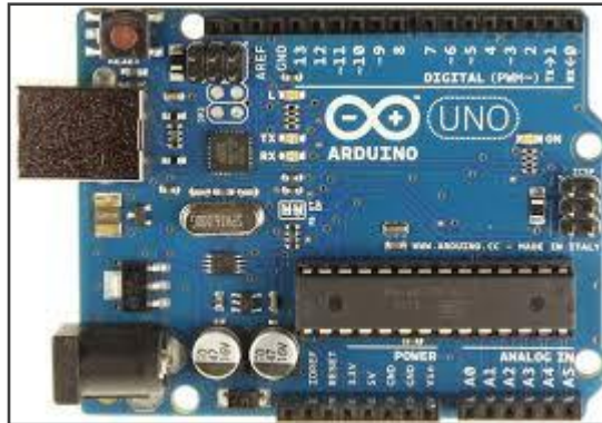
Figure 2: Arduino UNO board with Atmega328p microcontroller.
