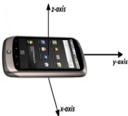
Fig 1 Three-axis diagram of the accelerometer.
