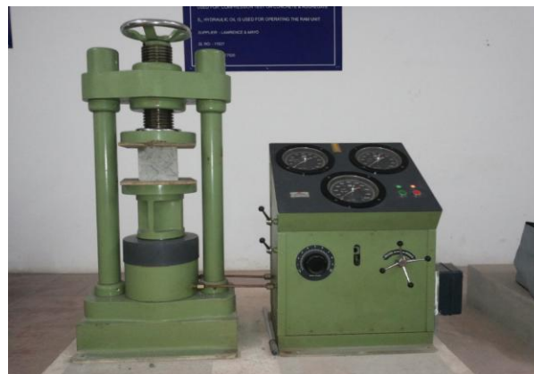
Fig. 1. Compression test on cube specimen.
