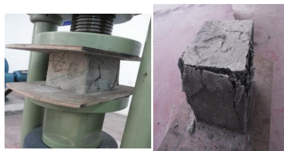
Fig. 2. Cube resistance to cracking due to binding of fibres.
