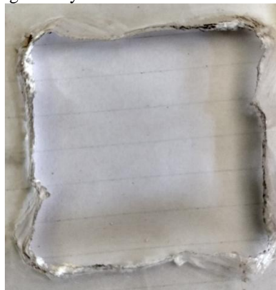
Fig8. Actual square hole drilled on acrylic
