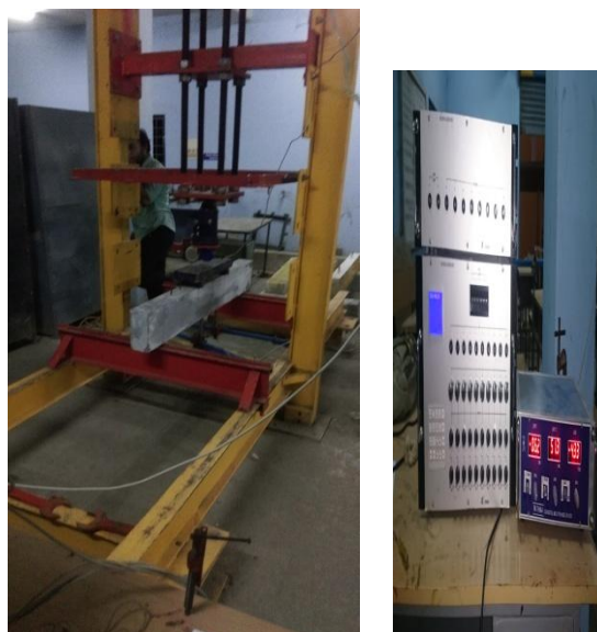
Figure.3 Testing set up of loading frame with data logger
