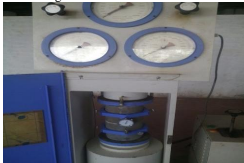
Fig 9 Using extensometer and compressive strength machine.
