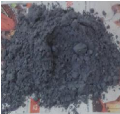
Fig 2:-RHA –Rice Husk Ash(RHA contains 85%-90% amorphous silica.)
