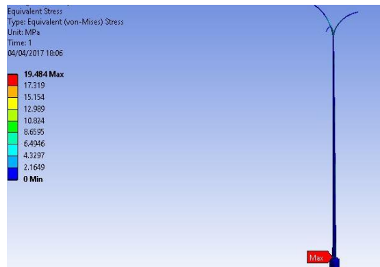
Fig.10: Stress diagram of hexagonal FRP pole
