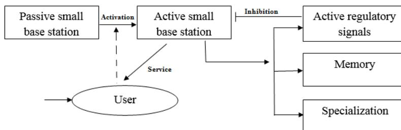
Fig 2: AIS-based SON approach for ultra-dense small cell network
