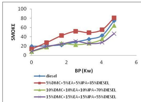
Smoke formation occurs at the extreme air deficiency. Air or oxygen deficiency is locally present inside the diesel engines. It increases as the air to fuel ratio decreases. Fig shows variation of smoke emissions for 15%, 30% & 45% oxy diesel blend. Since at high load, oxygen present in fuels leads to better combustion may take place inside the engine cylinder trying to reduce the smoke emissions. That 30 & 45% of oxy fuels smokes are lesser than the diesel
