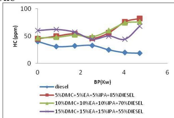
Hydrocarbon emission in diesel engine indicates that the quality of the fuel-air mixture and incomplete combustion during the combustion process. Fig.10.5 shows that the HC emissions at different load conditions for blending with different ratios and without blending. The study explored that the increase in HC emissions
