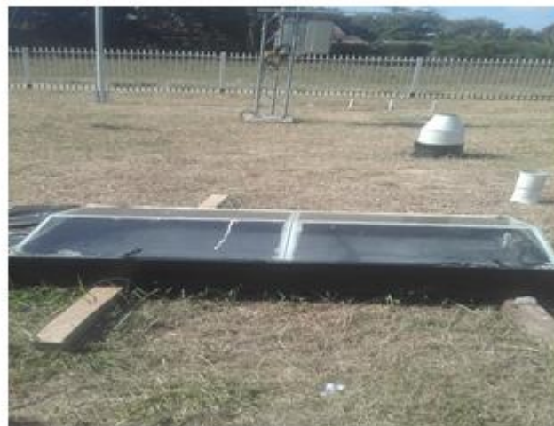
Figure 2: Double slope solar still in north south orientation
