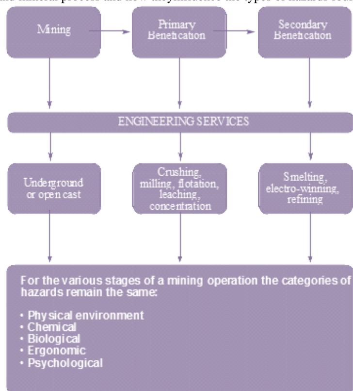
Figure 1: Illustrative flowchart for a mining operation
