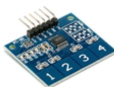
Figure 6: TTP224 4-ways capacitive touch sensor (12)
