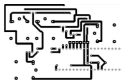
Figure 13: Soldered Side of the PCB (Bottom side)
