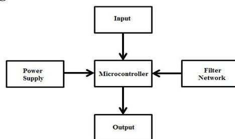
Figure 4: Block diagram of the developed system
