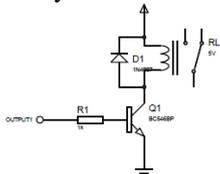
Figure 8: One channel output with relay driver
