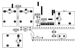
Figure 14: Component side of the PCB (Top side)
