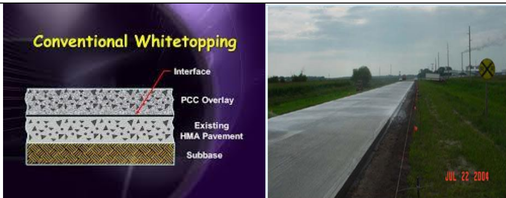
Fig 2.2 shows the conventional white topping
