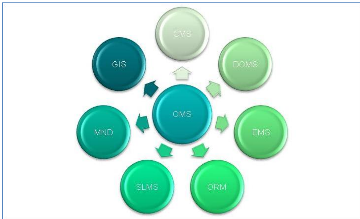
Figure 3: Outage management system (OMS) current architecture
