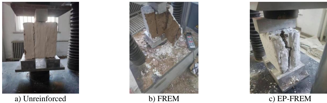
Figure 3: Shear failure pattern of adobe masonry
